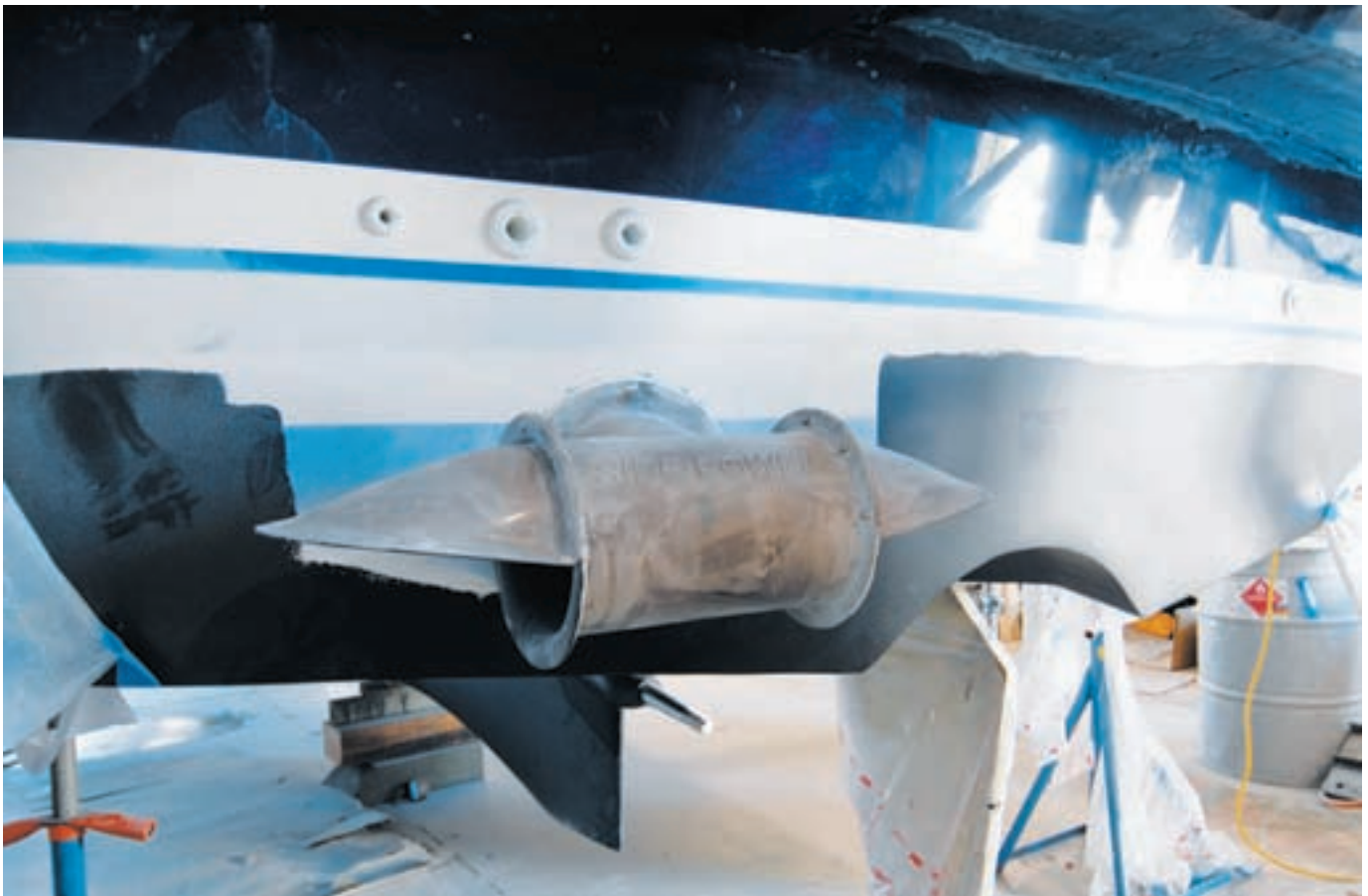
Side-Power stern thrusters are standard on the Fathom 40 and should ease the process of mooring the single-engine boat.
